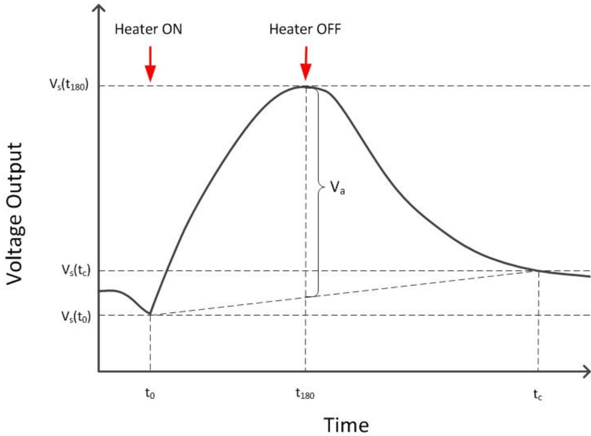
**Figure 2.** A conceptual plot of the voltage output ( $V_s$ ) from the sensor when performing a self-calibration. After the sensor response to self-heating ( $V_a$ ) is obtained, the *in-situ* correction factor ( $E_f$ ;  $V/Wm^{-2}$ ) for the plate is then estimated as:
