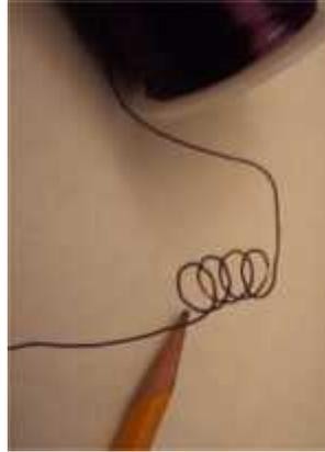
**Figure 2.** Bailing wire coiled around a pencil
