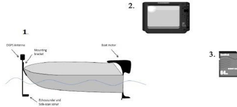
**Figure 3.** Bathymetric mapping system components. 1) Placement of sounder and transducer on the boat; 2) HumminBird main control panel; and 3) SD memory cards
