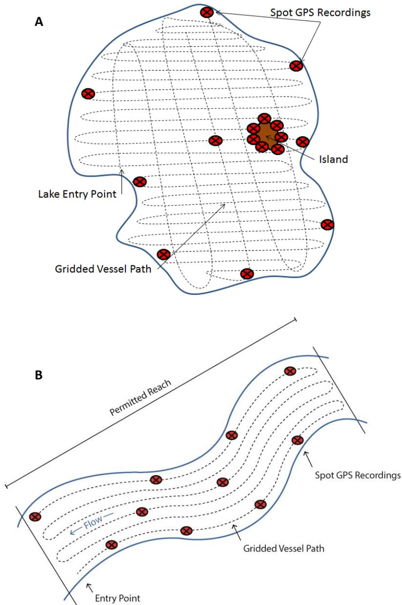
**Figure 10.** Schematic of gridded pattern undertaken in the vessel and approximate locations for (A) lake shoreline and island point GPS measurements as well as (B) non-wadeable stream GPS measurements. Note: grid lines should be approximately 20 m apart, figures are not to scale.
