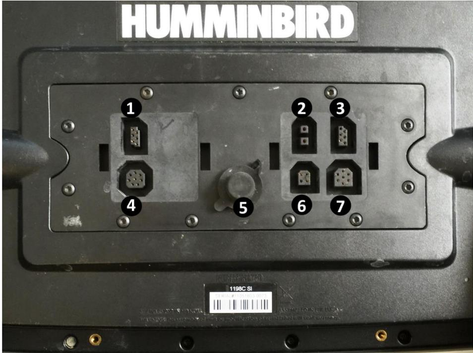
**Figure 5.** Rear view of the HumminBird control panel with connector details. 1) Video-Out (RS-232), 2) Power, 3) GPS/Communications, 4) Video Out, 5) Ethernet, 6) Temperature/speed, and 7) Transducer
