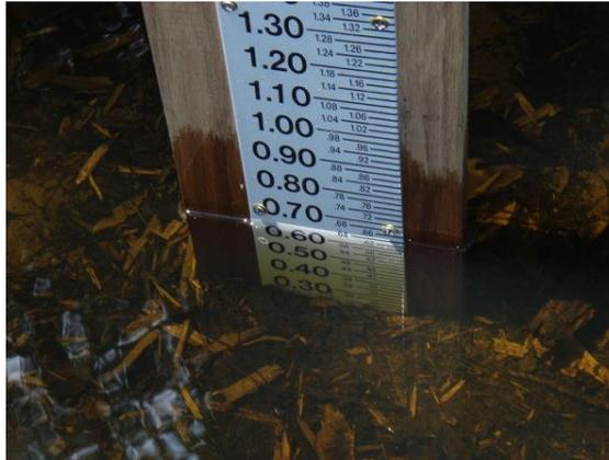
**Figure 7.** Example of a staff gauge. If conditions are wavy note the mean height.
