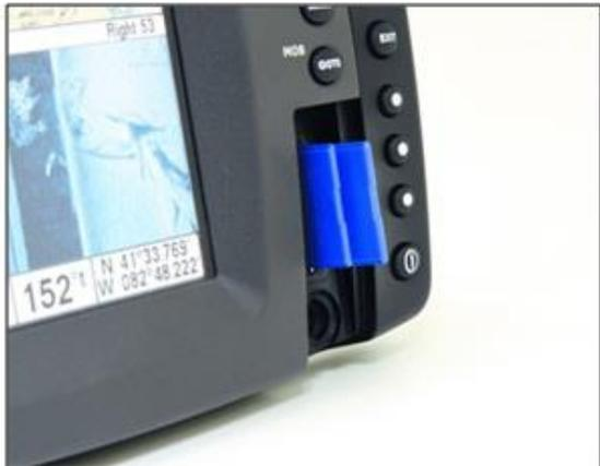
**Figure 6.** Insertion of SD cards in HumminBird card slot
