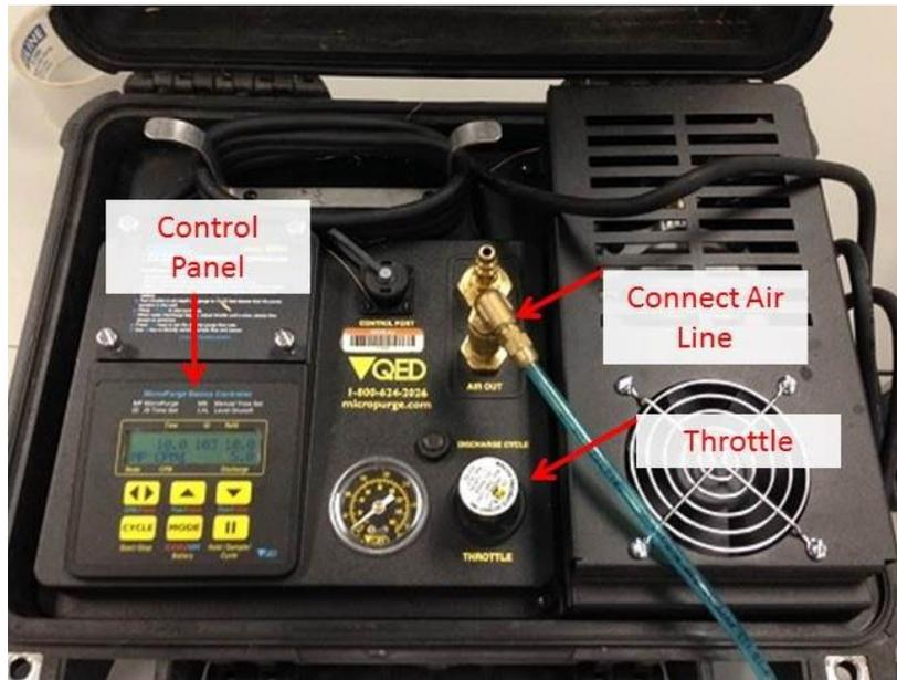
Figure 16. Attach blue air-line to controller
