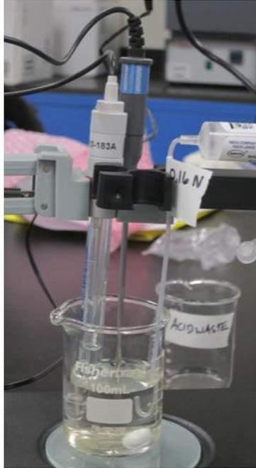
**Figure 25.** Image of titration set-up with digital titrator, stir bar, pH meter and temperature probe. Ensure nothing is touching the sides and bottom of the beaker or the stir bar
