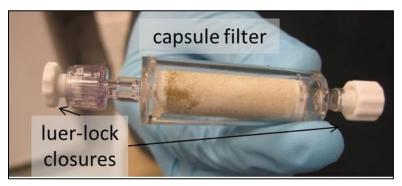
Figure 8. Capsule (Sterivex®) filter and luer lock closures
