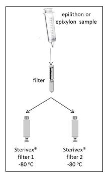
**Figure 11.** Schematic for benthic biofilm sampling via scrub slurry (SOP C).
