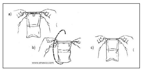
**Figure 13.** How to close a Whirl-pak® bag: a) hold the wire tabs; b) whirl the bag 3 complete revolutions (or fold the top over); and c) fold the wire ends over to close
