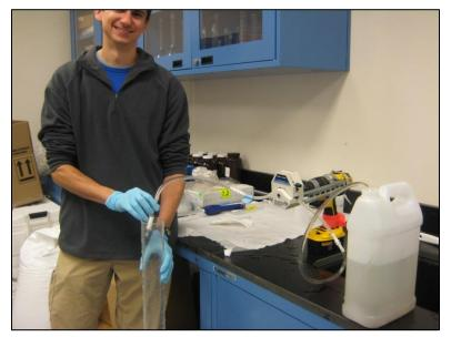
**Figure 7.** A field technician demonstrates pumping sample water out of the 4 gallon HDPE jug, through the peristaltic pump, the trough the Sterivex® filter, and into a graduated cylinder to measure the volume filtered.
