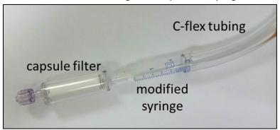
Figure 2. Filter adapter for peristaltic pump
